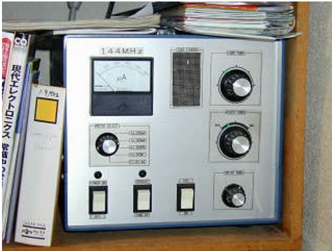
Front Panel : Multi-meter , Knobs and Tube Finder
