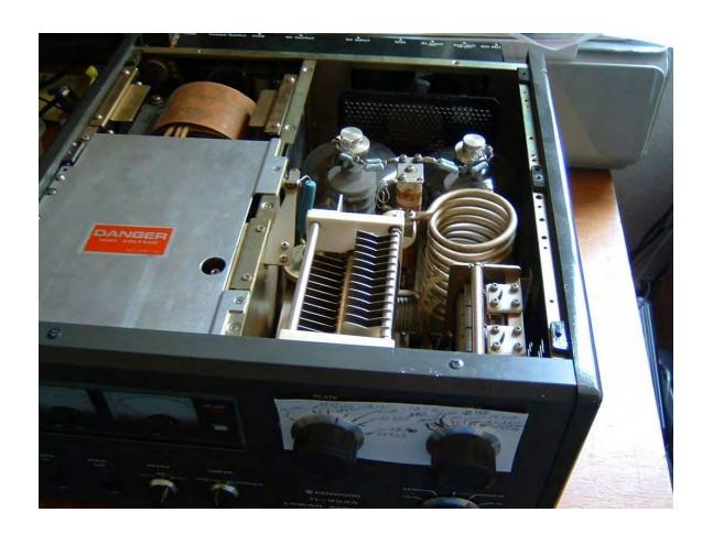
Remove the top cover and the RF cage shield cover. Turn the load capacitor fully counter clockwise.
