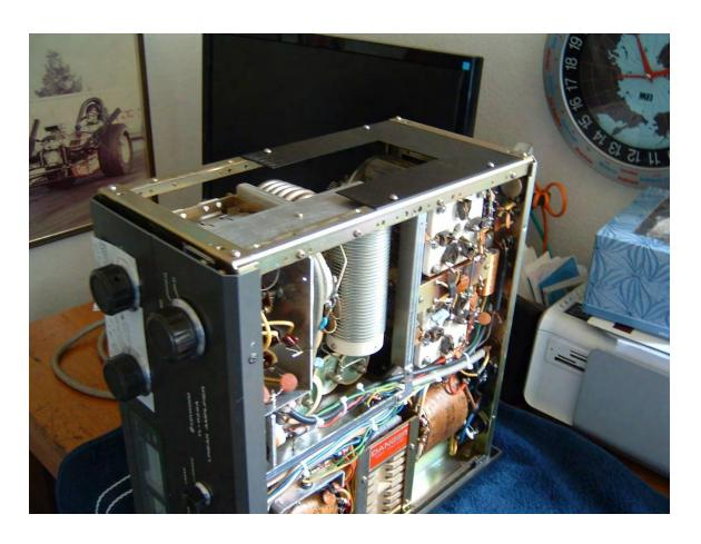
The side panel is removed to help with access to the upper switch contacts during removal and re-soldering.
