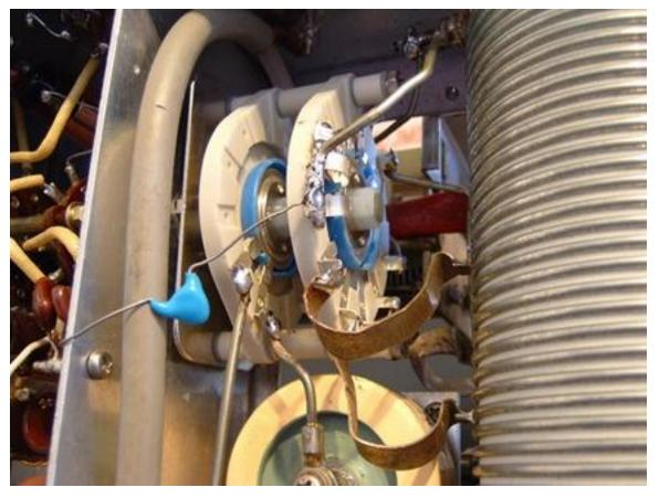
The finished switch Installed. Double check that the switch contacts are perfectly centered as the switch is rotated through the band positions. Time to put the covers back on!!
