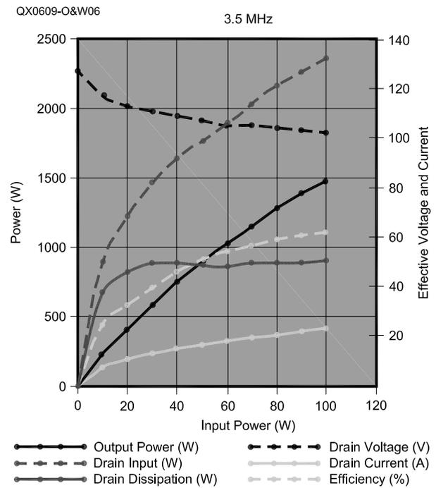
Figure 6 — This graph shows the amplifier characteristics on the 80-m band (3.5 MHz).
