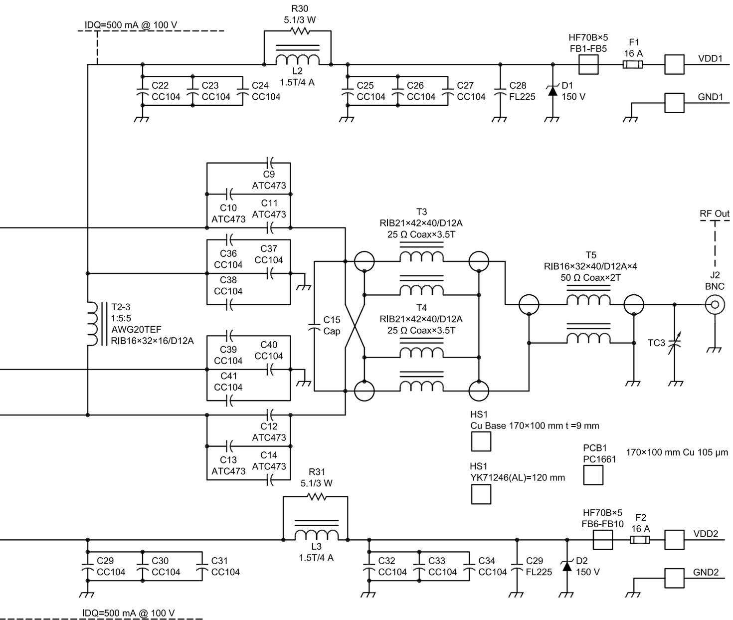
Figure 1 — Schematic diagram of the ARF1500 amplifier.
