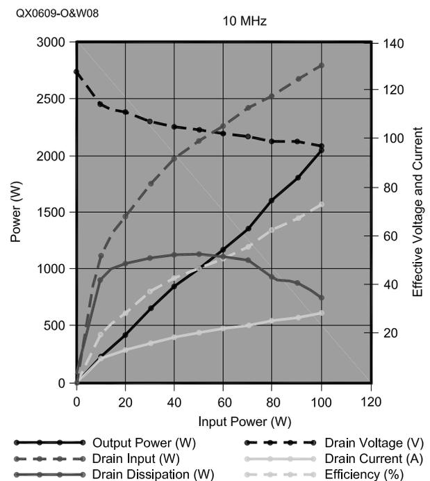
Figure 8 — This graph shows the amplifier characteristics on the 30-m band (10 MHz).
