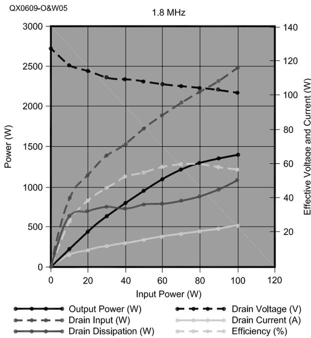
Figure 5 — This graph shows the amplifier characteristics on the 160-m band (1.8 MHz).
