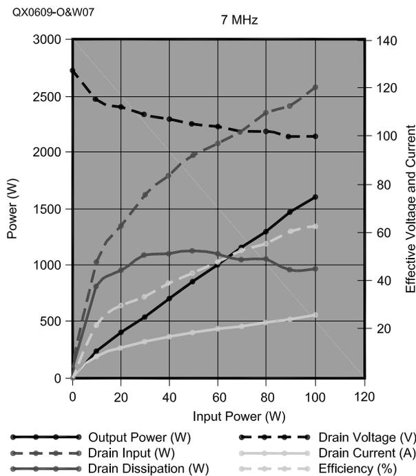
Figure 7 — This graph shows the amplifier characteristics on the 40-m band (7 MHz).
